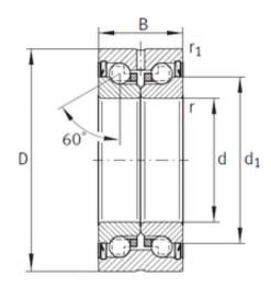
ZKLN0832-2Z Bearing 2D drawings and 3D CAD models
