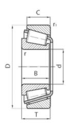
88,9 mm x 200 mm x 49,212 mm 88,9 mm x 200 mm x 49,212 mm Timken NP697931/NP241715 tapered roller bearings
