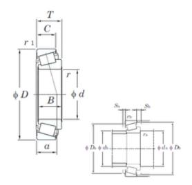
32 mm x 59 mm x 18 mm 32 mm x 59 mm x 18 mm KOYO HI-CAP ST3259 tapered roller bearings
