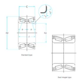
25 mm x 52 mm x 42 mm 25 mm x 52 mm x 42 mm SNR FC41950 tapered roller bearings
