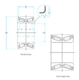
35 mm x 62 mm x 52 mm 35 mm x 62 mm x 52 mm NTN 4T-CRI0778 tapered roller bearings
