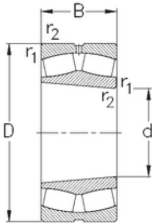
110 mm x 200 mm x 53 mm 110 mm x 200 mm x 53 mm NKE 22222-E-K-W33 spherical roller bearings
