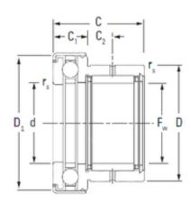
NAXK15Z Bearing 2D drawings and 3D CAD models
