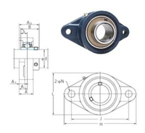
UCFL205E Bearing 2D drawings and 3D CAD models
