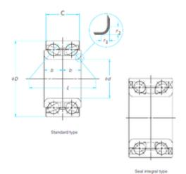
36 mm x 76 mm x 29,2 mm 36 mm x 76 mm x 29,2 mm SKF BA2B440190C angular contact ball bearings
