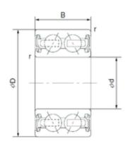
32 mm x 55 mm x 23 mm 32 mm x 55 mm x 23 mm CYSD 46/32-2AC2RS angular contact ball bearings
